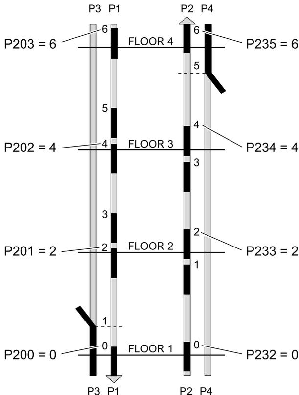
**Figure 9.3 Example Floor Position**
