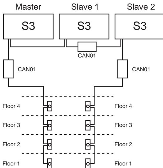
**Figure 22.3 CAN01 Redundancy 2**
